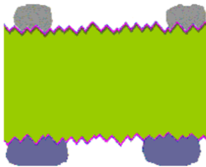
g) Print-screening Ag paste on front surface of the cell (a layer about 30-50 \mu\text{m} thick)
