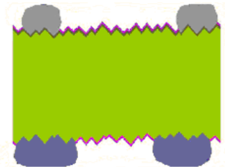
h) Contact sintering at temperature about 800°C, realisation ohmic contacts, edge grinding.
