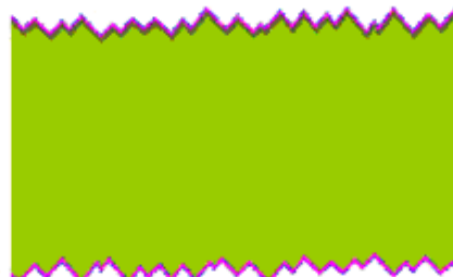
e) Antireflection coating with silicon nitride layer of thickness about 75 \mu\text{m} , both sides
