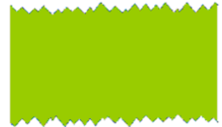
c) Silicon wafer after surface texturing by anisotropic etching in KOH (NaOH)
