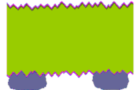
f) Print-screening Al + Ag paste on back surface of the cell (a layer 30-50 \mu\text{m} thick)
